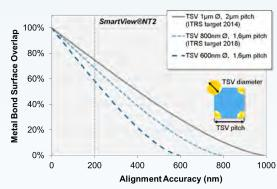
Calculated surface overlap of metal TSVs for hybrid bonding as a function of wafer-to-wafer alignment accuracy. Comparison of ITRS roadmap relevant TSV pitches and diameters reveal, alignment accuracy of better than 200nm ( $3\sigma$ ) is needed to achieve 60% and more TSV overlap for hybrid bonding.
